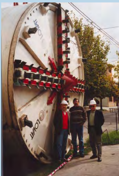
TBM – Shield, for excavation of soils in urban environment
